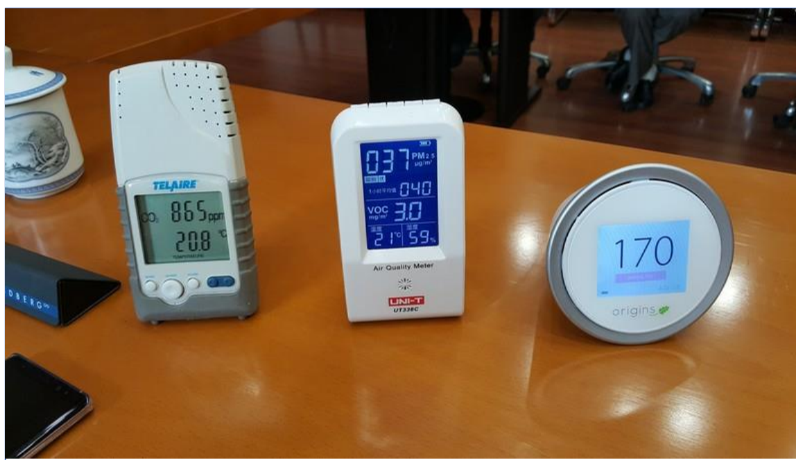
Figure 70 Measured CO 2 , VOC and PM 2.5 AQI Level in UNICEF
